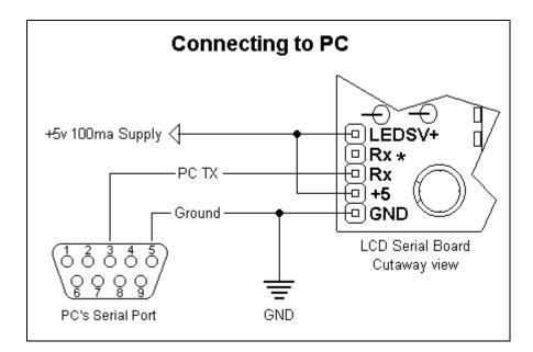
Note: Never connect LEDSV+ to +5 on the BX-24! The BX-24 +5 regulator cannot supply enough current to power the LCD backlight and will overheat.
