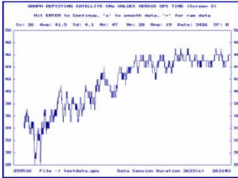
Figure 9.3: C/No Values (Y axis) Versus GPS Time (X axis)
