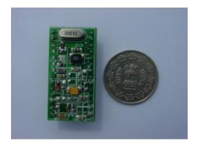
**RFID Reader Module**, are also called as interrogators. They convert radio waves returned from the RFID tag into a form that can be passed on to Controllers, which can make use of it. RFID tags and readers have to be tuned to the same frequency in order to communicate. RFID systems use many different frequencies, but the most common and widely used & supported by our Reader is 125 KHz.
